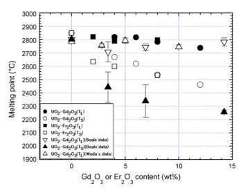
Fig. 5. The melting points of UO2-Gd2O3, UO2-Er2O3 and UO2 fuels.
