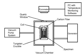
Fig. 1. Schematic diagram of the apparatus for measuring the melting temperature.
