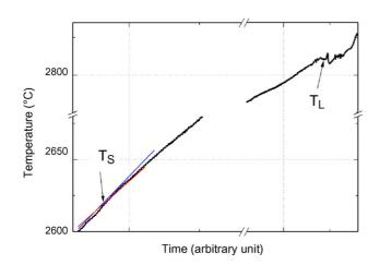
Fig. 4. A temperature–time plot showing the solidus and liquidus temperatures of  $UO_2-6$  wt%  $Gd_2O_3$  by the thermal arrest method.
