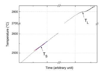
Fig. 3. A temperature–time plot showing the solidus and liquidus temperatures of  $UO_2-8$  wt%  $Er_2O_3$  by the thermal arrest method.
