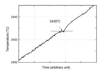
Fig. 2. A temperature–time plot showing the melting point of  $Gd_2O_3$  as a reference sample.
